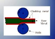
Fig: The roll bonding or cladding process
