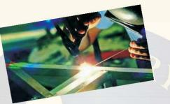
than just the surface of the material has been heated. When an interpass temperature is specified, the weld area must be inspected prior to depositing the next weld bead.
