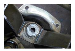
The 20mm thick sheet was MIG welded with a single V groove. However, the non uniform cooling issue and the residual stress thus formed led to angular distortion in the welded plate. The distortion though was very little, but none the less that gave me an out of proportion finished component.
